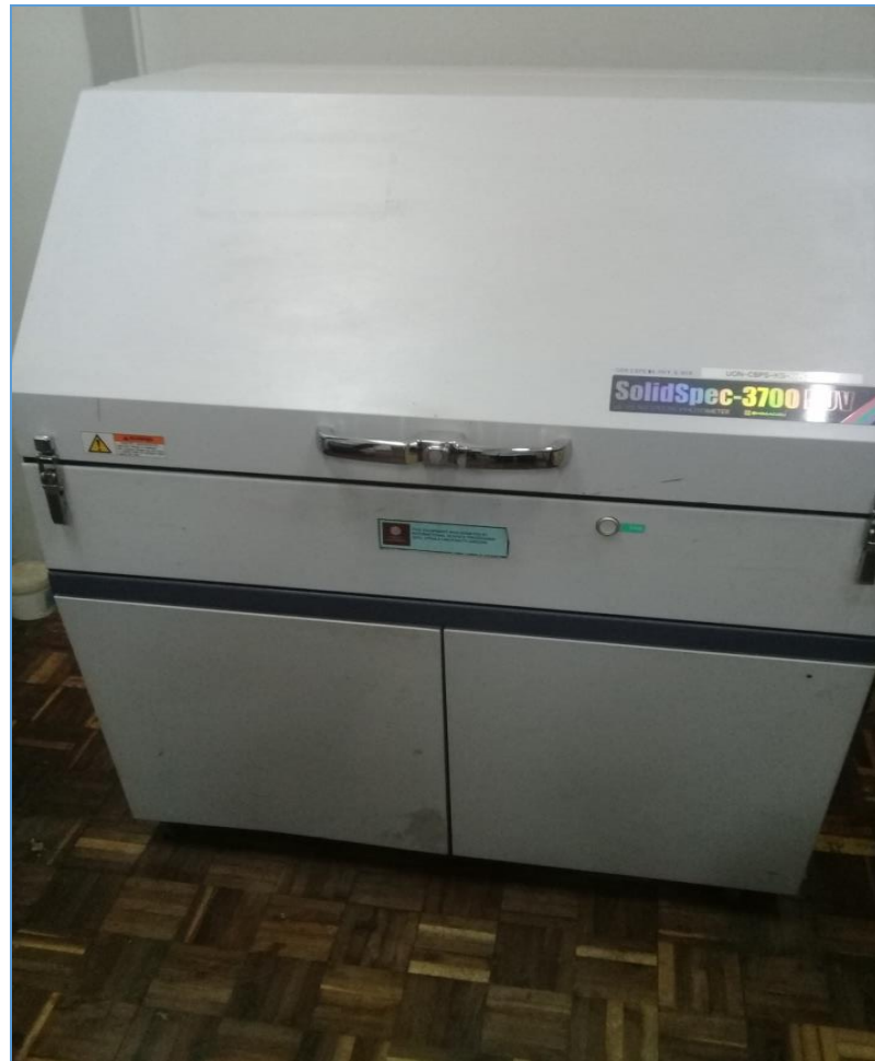
Figure 4.4: DUV 3700 solid spectrophotometer
