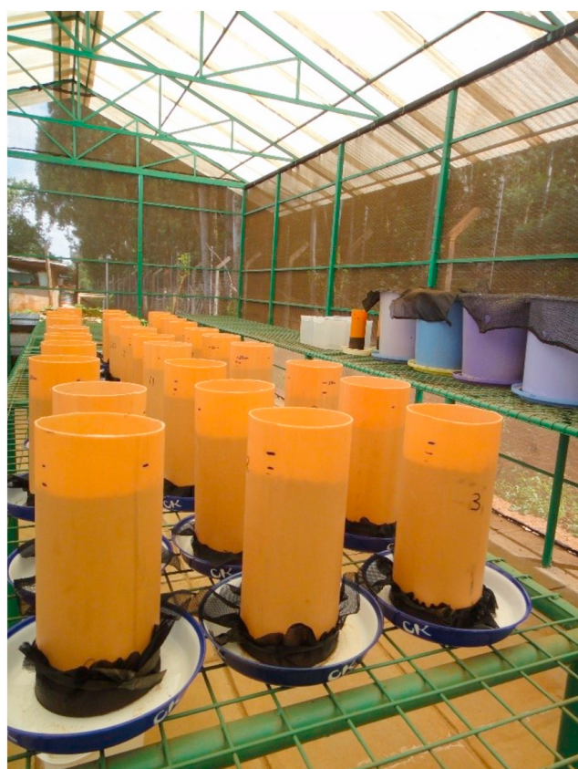
Fig. 1. Microcosms with muslin cloth fitted at the base on water filled plates to allow for wetting by capillary action.
