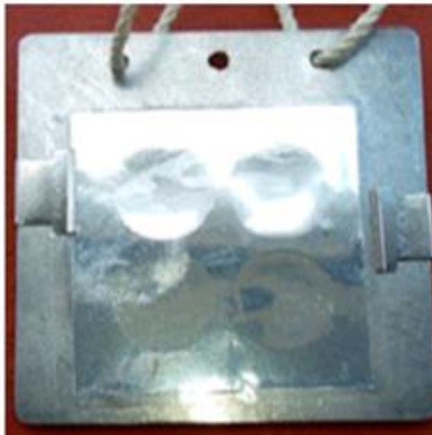
Plate 3.2: An overview of thoron progeny monitor
