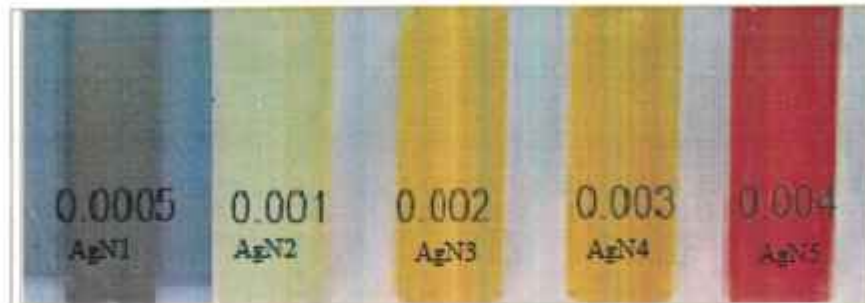
Figure 4.6: Distinctive colour of different sized silver nanoparticles
