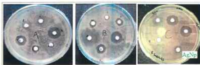
Figure 4.15: Zones of inhibition for AgNps with different particles size against B. subtilis done in triplicate
